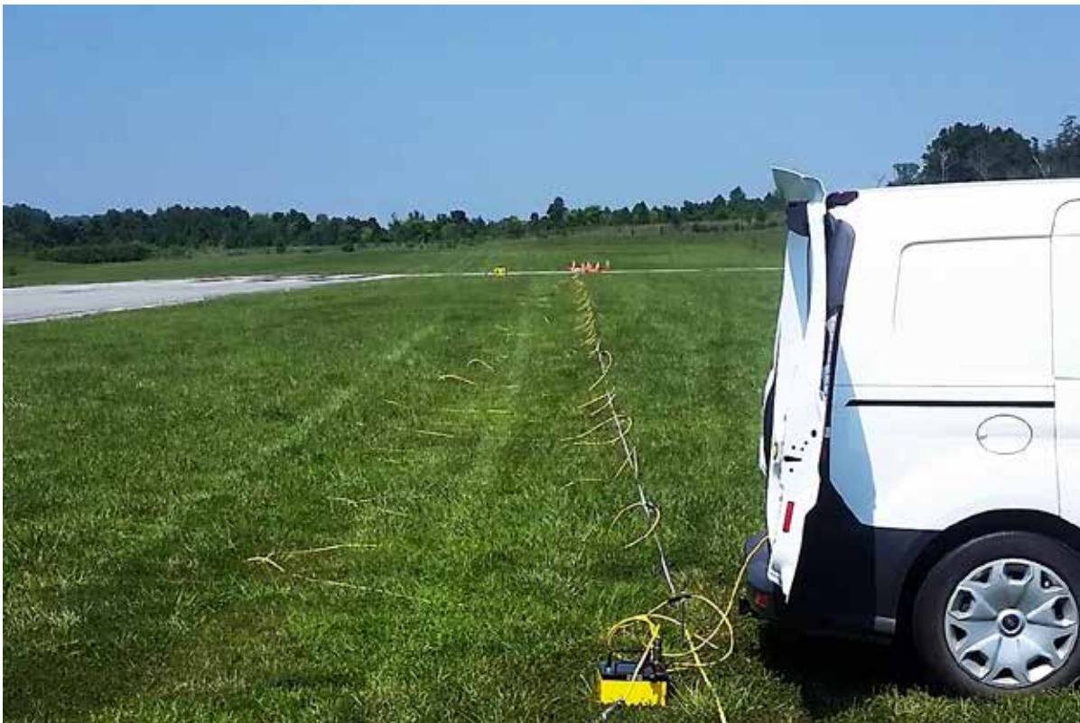
Figure 11: Photo of ERT layout located east of the runway (view to the north).
